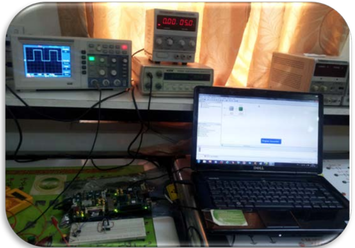
Figure (9): Hardware components for downloading the bit stream into the training kit.
